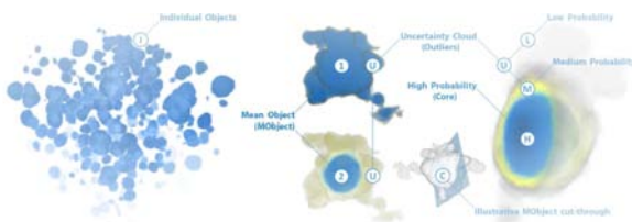
Figure 1: MObjects: The individual objects on the left side are combined to a Mean Object, and a cut through of it on the right side. The blue core of the object depicts a high probability of voxels belonging to the MOObject. This core is surrounded by the yellow medium probability layer which together with the outermost low probability layer forms the uncertainty cloud. ©2013 IEEE. Reprinted, with permission, from [RGK*13].
